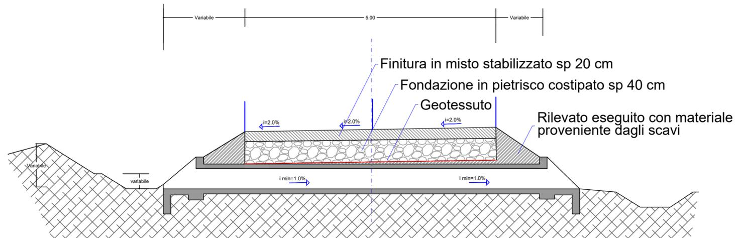
DETTAGLIO MANUFATTO IMBOCCO/SBOCCO\_SCALA 1:50
