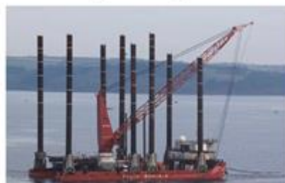
d) Jackup barge
