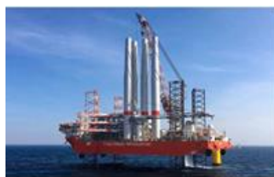
e) Purpose-built jackup vessel
