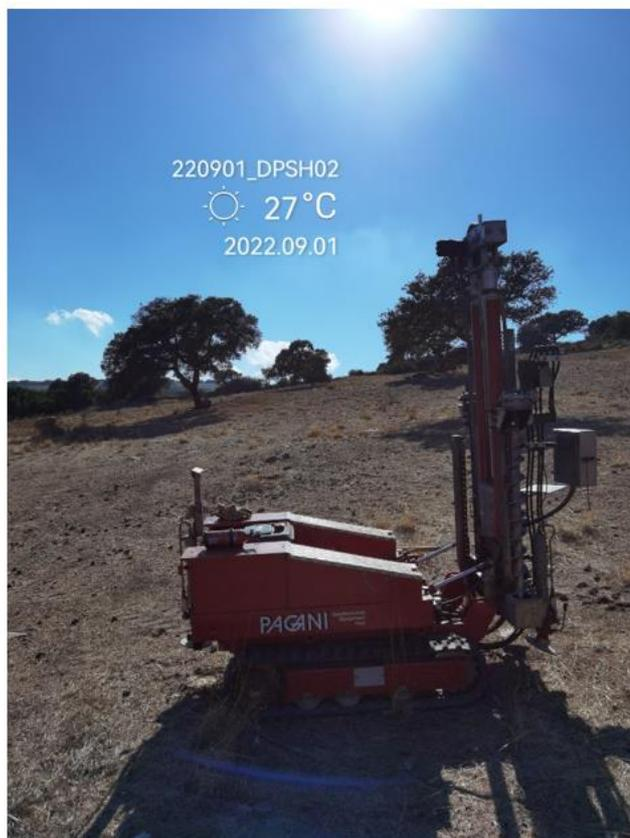
**Foto 1 e 2 Prova penetrometrica 220901\_DPSH01 e 22901\_DPSH02**
