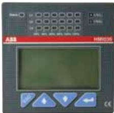
This can be used with all the protection releases fitted with dialogue, it is designed to be installed on the front of the panel. It consists of a graphic display where all the measurements and the release alarms/events are displayed. Thanks to its high level of precision, the device can replace the traditional multi-meters without the need of current/voltage transformers. L'HMI030 is connected directly to the protection release by means of a serial line and requires a 24 V DC power supply.
