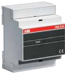
The VM210 accessory, combined with the protection devices, provides different measurements of the electrical values of the plant. It is able to provide measurements relative to a maximum of 5 electronic releases. The connection distance between the module and the release is a maximum of 15 metres; for distances greater than 1 metre, it is necessary to use a shielded multi-pole connection cable.
