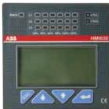
Can be used with all the protection releases fitted with dialogue, is designed to be installed on the front of the panel. It consists of a graphic display where all the measurements and alarms/events of the release are displayed. Thanks to its high precision, the device can replace traditional multi-meters without the need of current/voltage transformers. The HMI030 is connected directly to the protection release by means of a serial line and requires a 24 V DC power supply.
