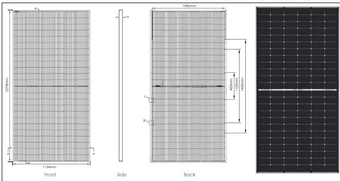
FIGURA 6: PANNELLO FV PARI A 570 WP CON DIMENSIONI 2278 X 1134 X 30 MM
