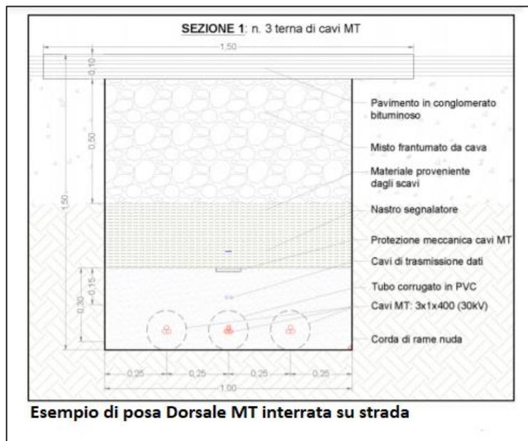
FIGURA 3: ESEMPIO TIPOLOGIA DI POSA PREVISTA TRA LA CABINE DI CONSEGNA E LA SE TERNA
