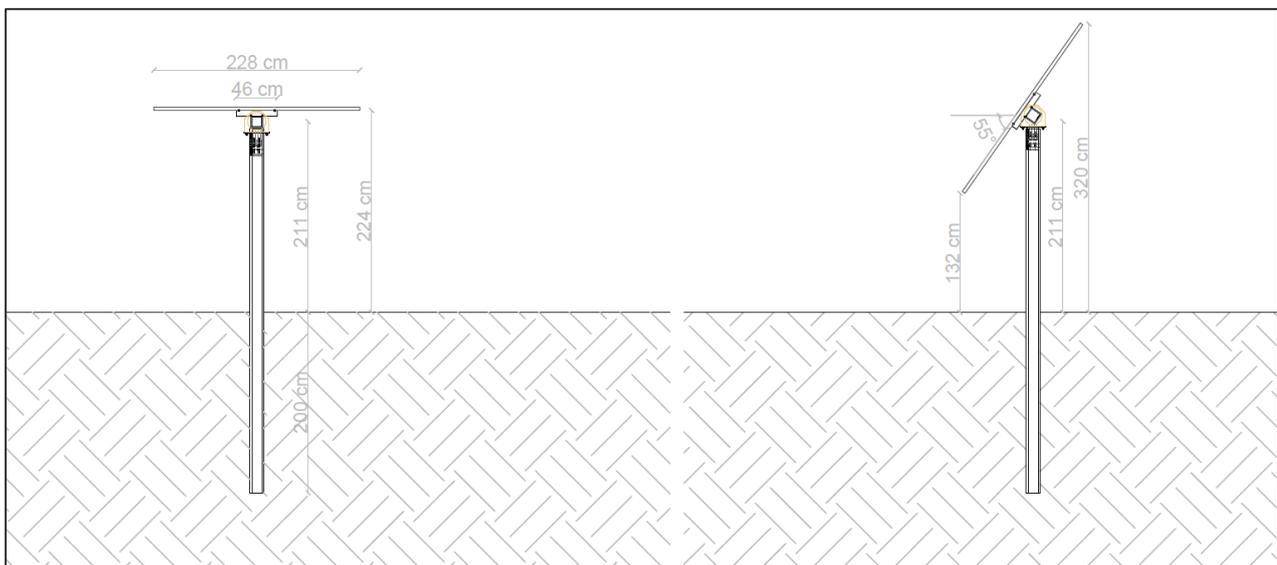
FIGURA 2: SCHEMA TIPO TRACKER AD ASSE VARIABILE
