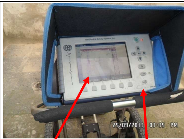
Software RADAN. SIR 3000 Controller.
