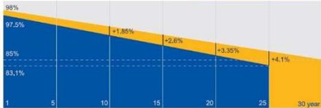
■ Bifacial double glass module linear power warranty    ■ Standard module linear power warranty
