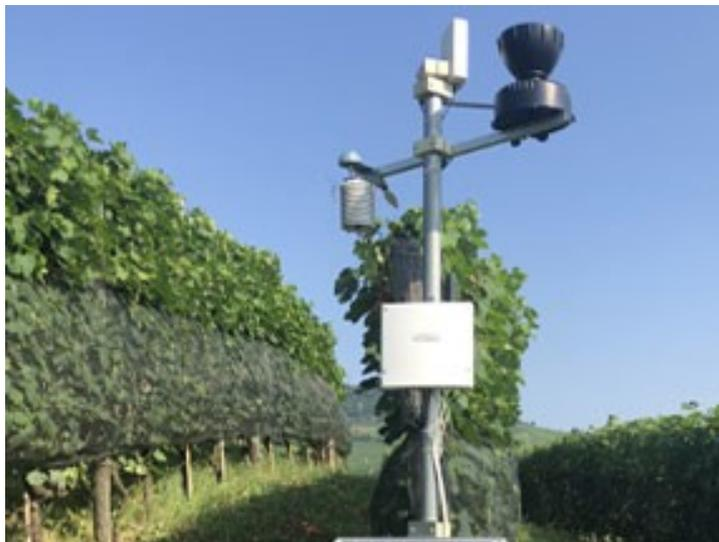
Figura 13-1 – Centralina meteorologica
