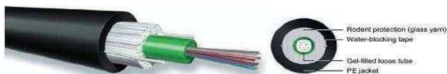
Figure 1: Fibre optic cable (cross section)
