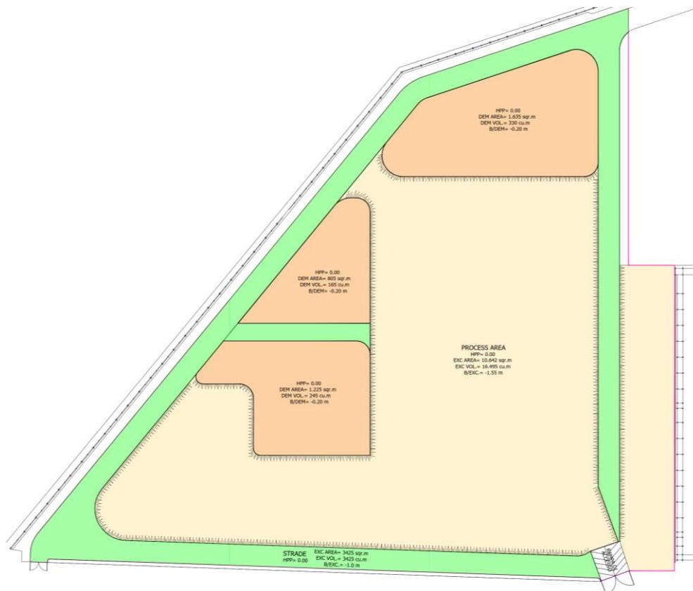
Figura 4 Pianta scavi Steam Reforming
