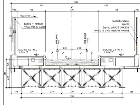
SEZIONE TIPO CON TRAVI INCORPORATE-Scala 1:100
