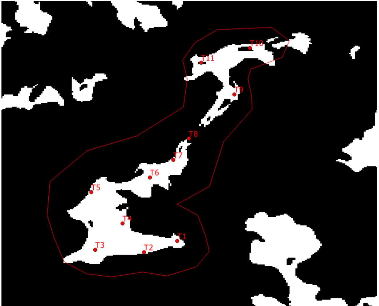
Figure 2.4: Wind constraints map at 100 m AGL with San Niccolò boundary in red (all sectors considered). White denotes areas which are viable for turbine placement.
