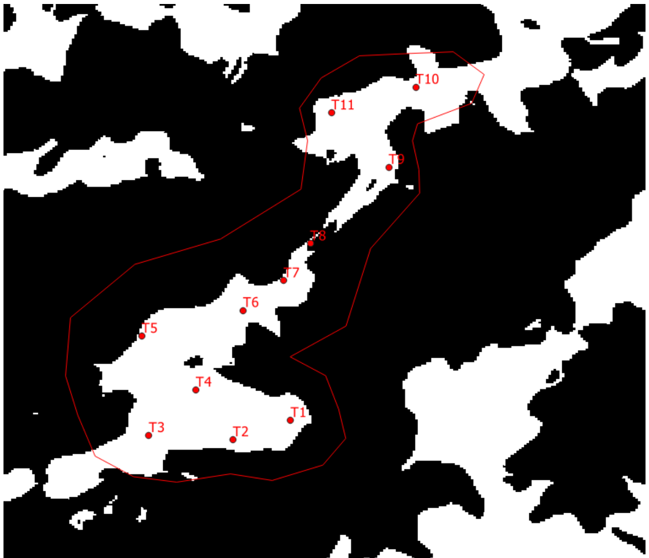
Figure 2.5: Wind constraints map at 100 m AGL with San Niccolò boundary in red (prevailing sectors considered). White denotes areas which are viable for turbine placement.
