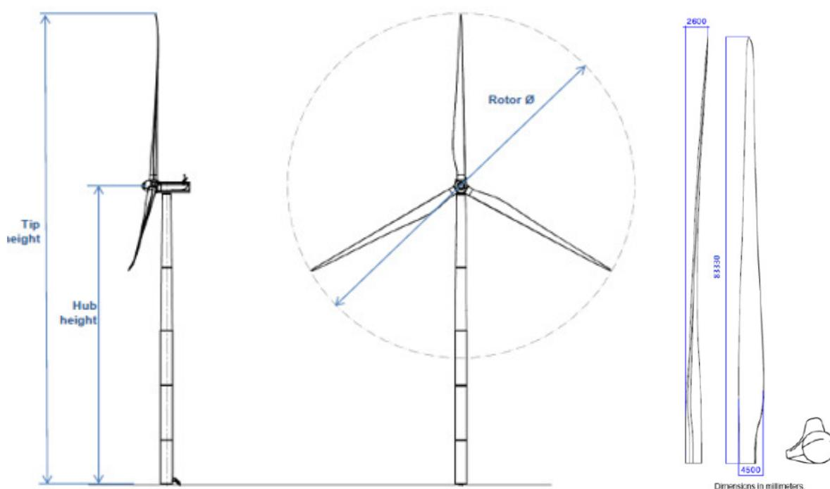
Tip height=220m; hub height=135m; rotor diameter=170m; blade length=83.33m
