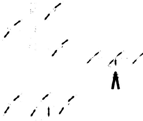
**Strain poles with one conductor above the crossarm. Risk high (see also Fig. 3):**
