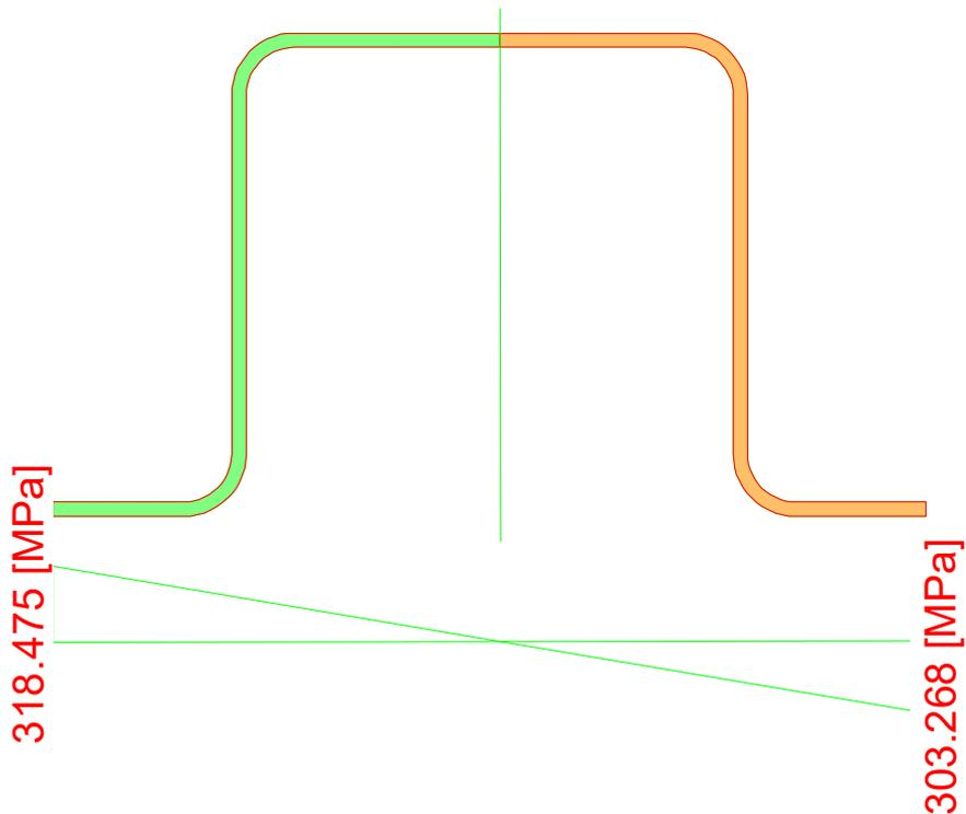
$$\sigma_{\max} = 318,4 \text{ N/mm}^2 < \left( \frac{f_{y,k}}{\gamma_{m0}} \right) = \left( \frac{355}{1,05} \right) = 338,1 \text{ N/mm}^2$$
