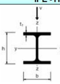
$$\frac{V_{Ed}}{V_{c,Rd}} \leq 1,0 \quad V_{c,Rd} = \frac{A_v (f_{yk} / \sqrt{3})}{\gamma_{M0}} \quad A_v = A - 2bt_f + (t_w + 2r)t_f$$
