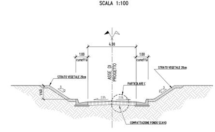
PARTICOLARE MARGINE TIPO IN RILEVATO – MARGINE ESTERNO
