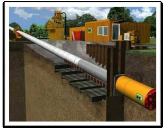
Figure 4-11. Schema tecnica "Microtunneling"
