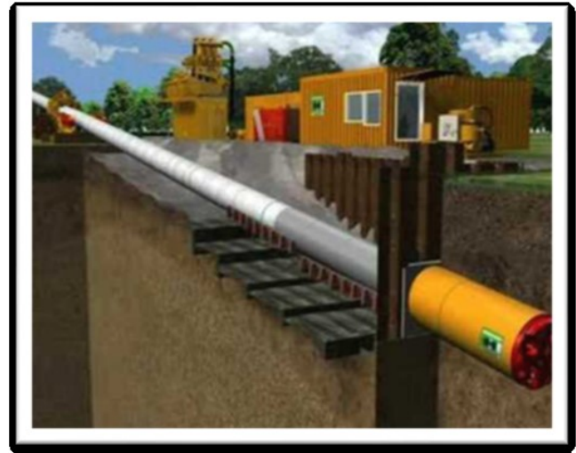
Figure 2-11. Schema tecnica "Microtunneling"
