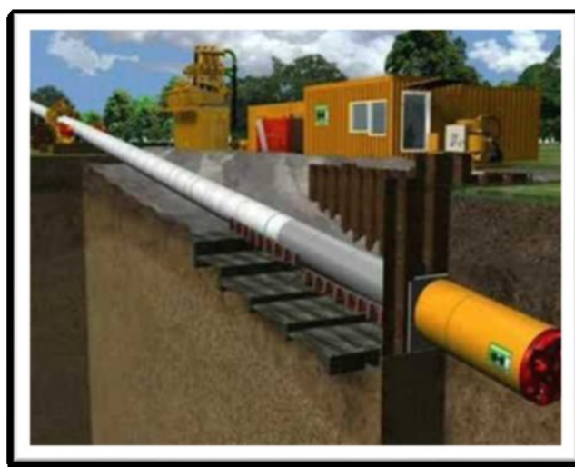
Figure 2-11. Schema tecnica "Microtunneling"
