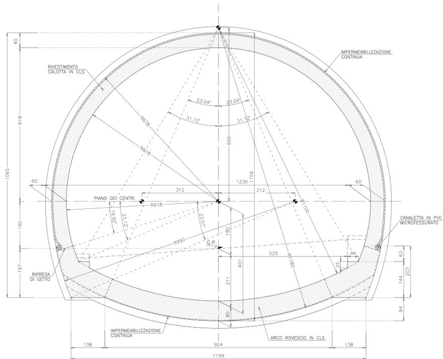
SEZIONE TRASVERSALE (MAX) TIPO C2VP 1-2-3-4
