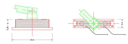
PARTICOLARE SISTEMA TIPO "RDS" ABBINATO A MICROPRISMI
