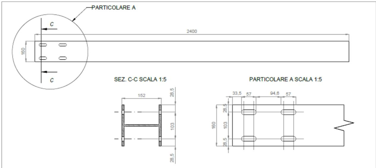
DETTAGLIO 5 PROFILO A Z 150x50x20 - MATERIALE S355JR SCALA 1:10
