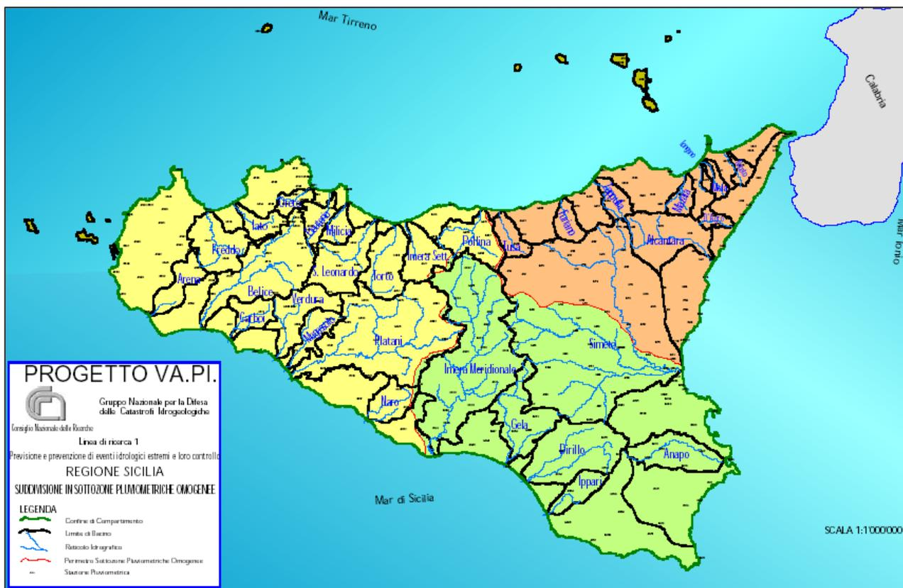
FIGURA 5.2.1- SUDDIVISIONE IN SOTTOZONA PLUVIOMETRICHE OMOGENEE: A (GIALLO), B (ARANCIO), C (VERDE).
