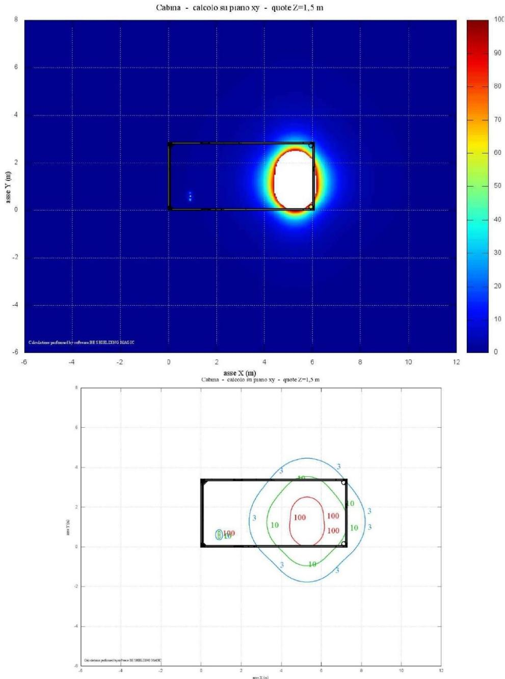
Figura 31: PS (SMA SC4200 UP), h = 1,5 m, mappa 2D e curve isolivello
