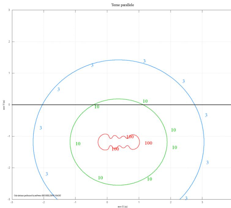
Figura 16: Anello PS, 4 terve, curve isolivello
