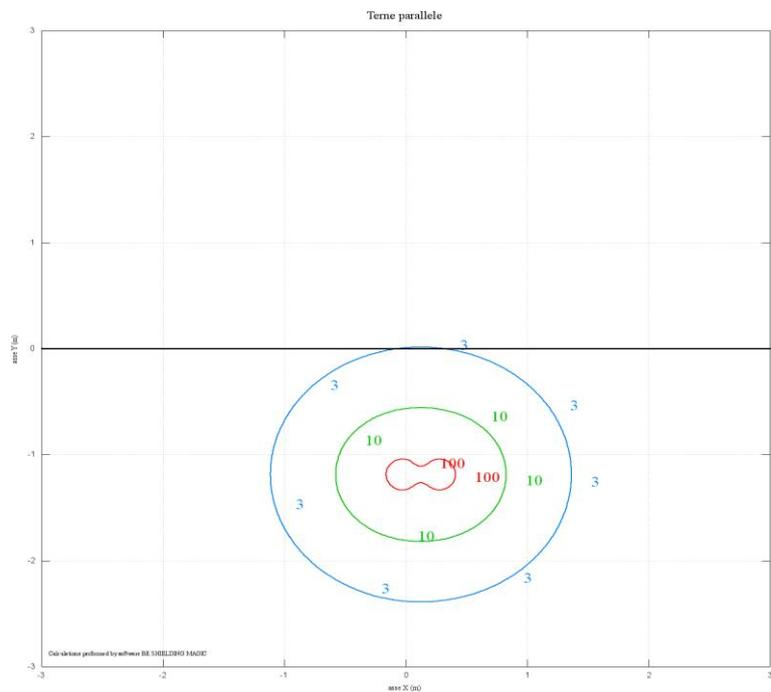
Figura 22: Anello SPS, 2 terre, curve isolivello
