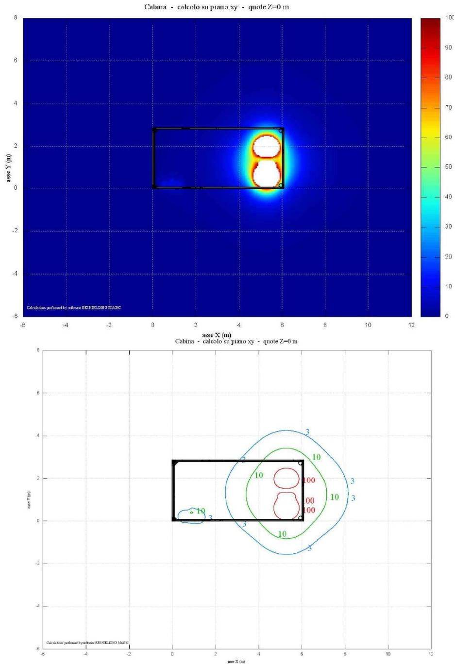
Figura 27: PS (SMA SC2660 UP), h = 0 m, mappa 2D e curve isolivello
