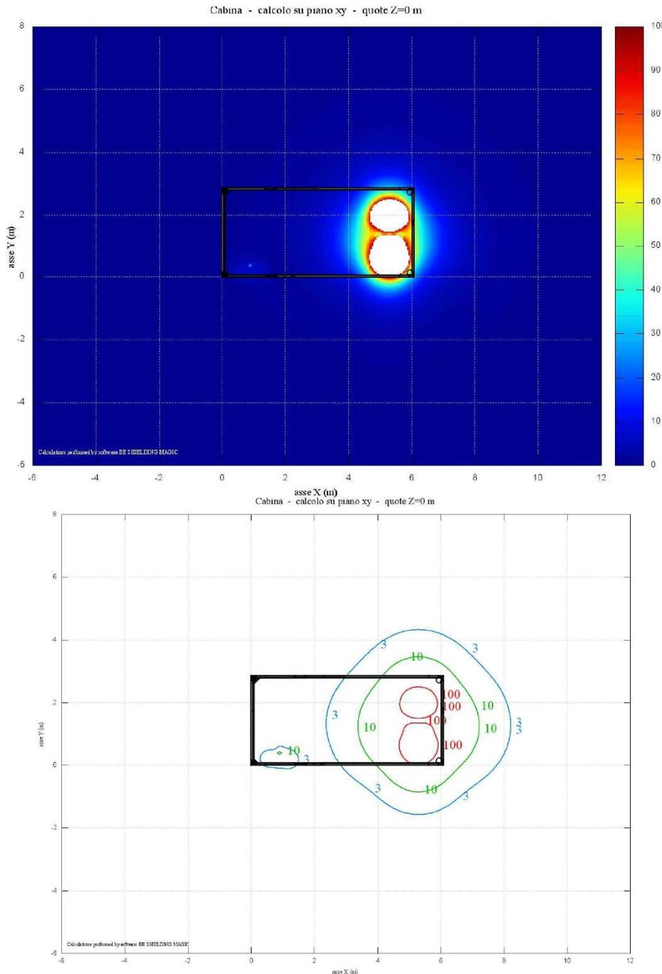
Figura 30: PS (SMA SC4200 UP),  $h = 0$  m, mappa 2D e curve isolivello
