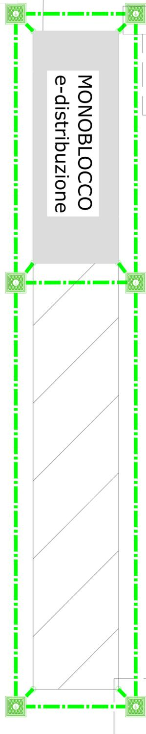
COLLEGAMENTO ALLA RETE ELETTROSALDATA DEL BASAMENTO DEI MONOBLOCCHI
