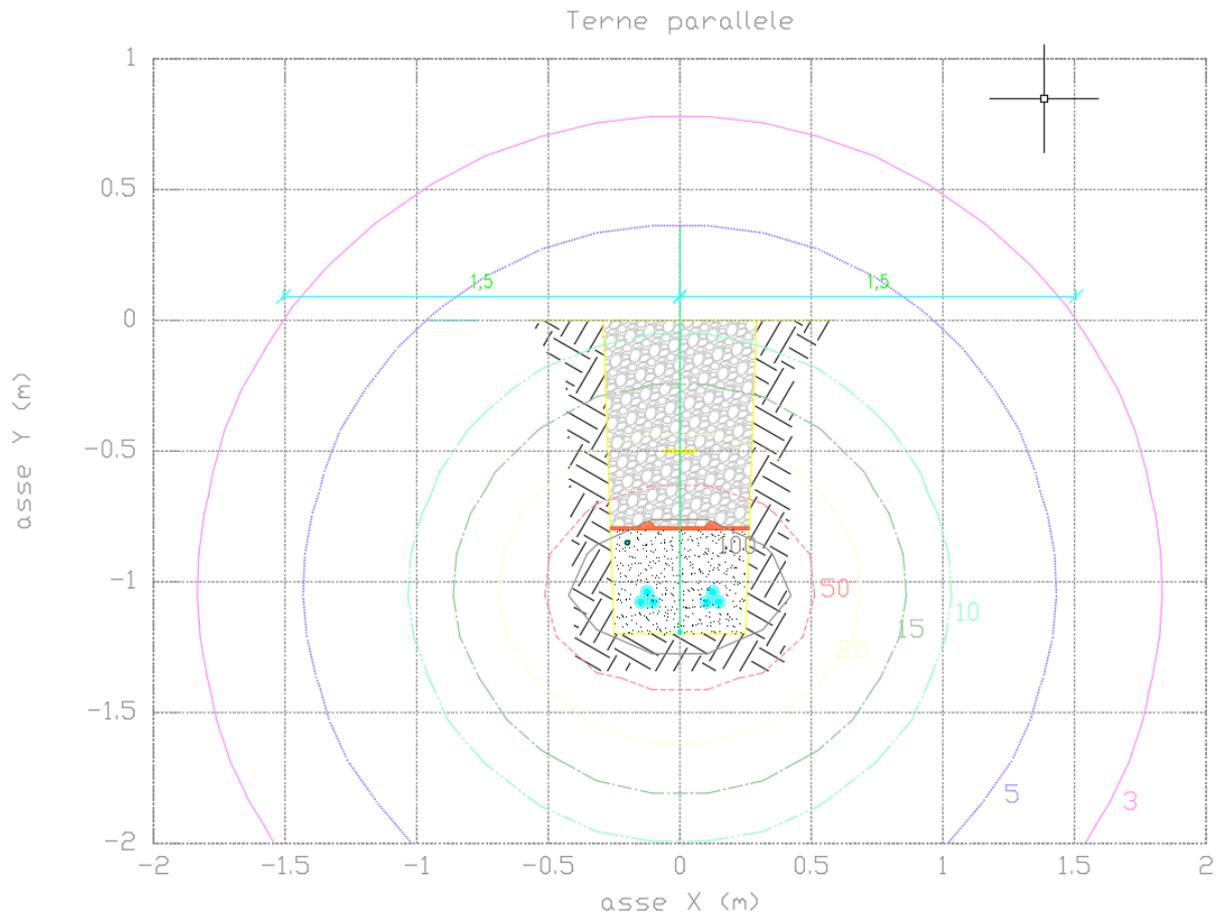
Calculations performed by software BE SHIELDING MAGIC
