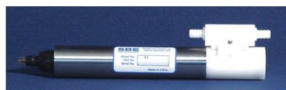
**Temperature response** and corrections are dramatically improved. The largest source of error in profiling applications is nearly eliminated, and the equilibration 'wait time' at the beginning of a profile is reduced to seconds. Profiling accuracy in gradients is dramatically improved.
