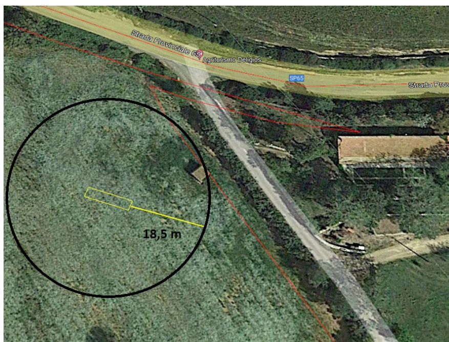
Figura 10 – DPA Power Station
