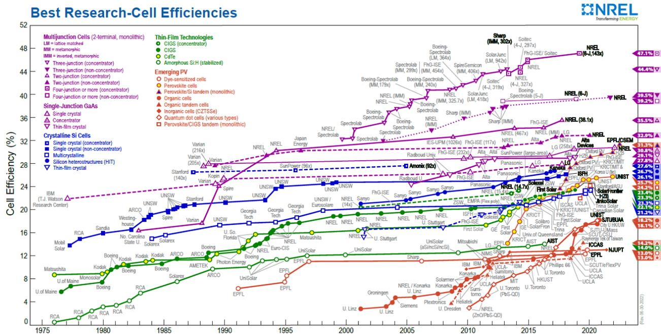
Figura 4.4 – Progressi della ricerca in termini di efficienza delle celle FV (fonte United States National Renewable Energy Laboratory <https://www.nrel.gov/pv/assets/pdfs/best-research-cell-efficiencies-rev220630.pdf>)
