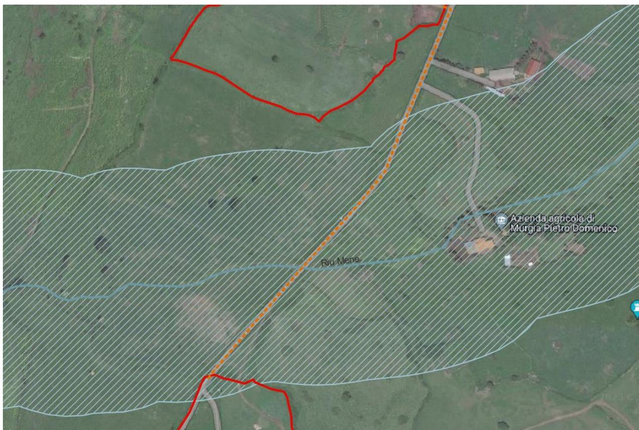
FIGURA 9 – PARTICOLARE: INTERFERENZA TRA CAVIDOTTO E FASCIA 150 M DAL RIU MENE – PASSAGGIO SU VIABILITÀ ESISTENTE
