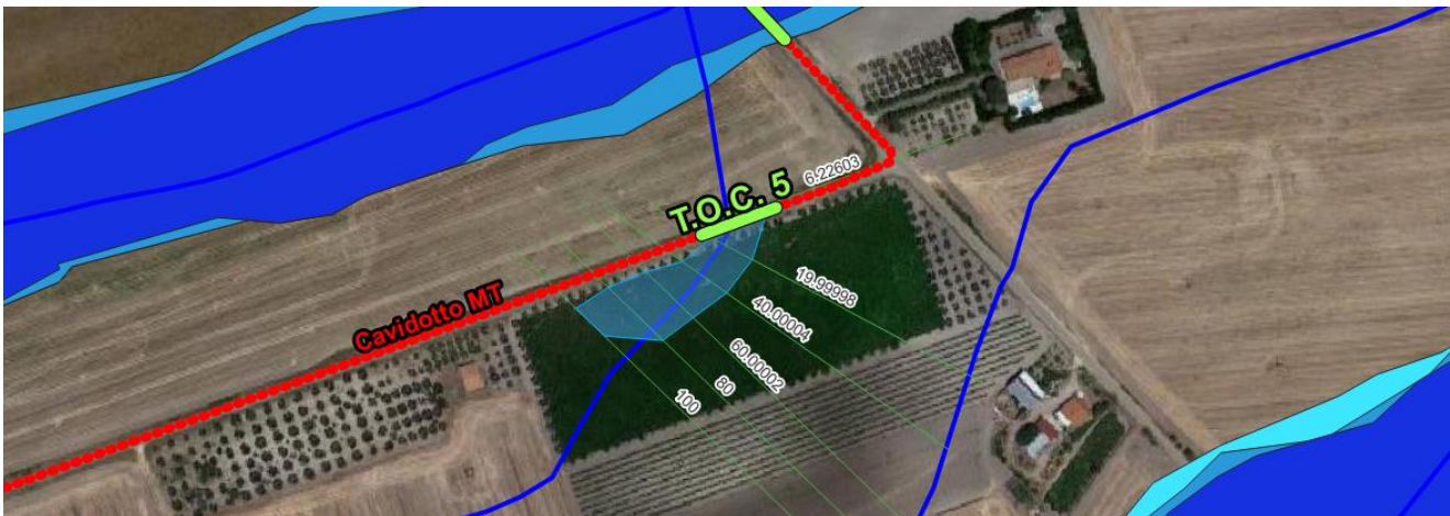
Attraversamento in T.O.C.
