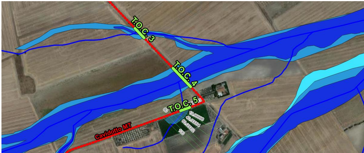
Attraversamento in T.O.C.
