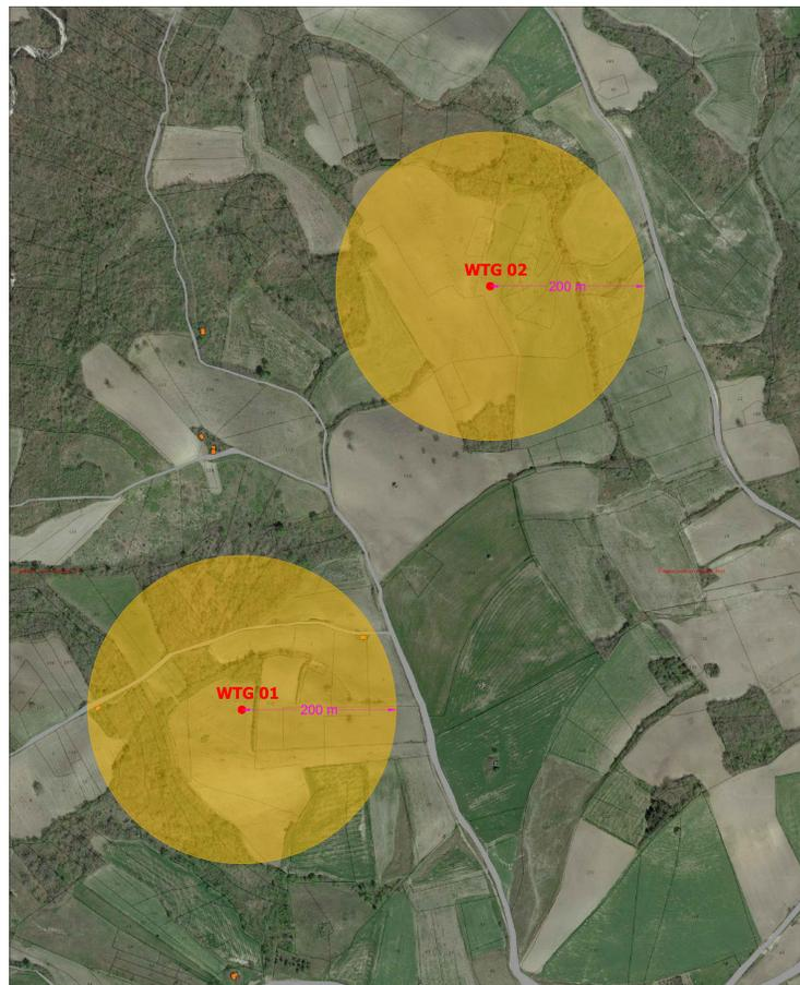
BUFFER DI 200 m RISPETTO A CIASCUNO DEGLI AEROGENERATORI WTG 01 E WTG 02
