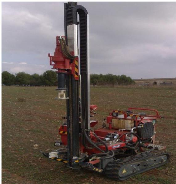
**FIGURA 8 - MACCHINA BATTIPALO PER INFISSIONE PALI.**
