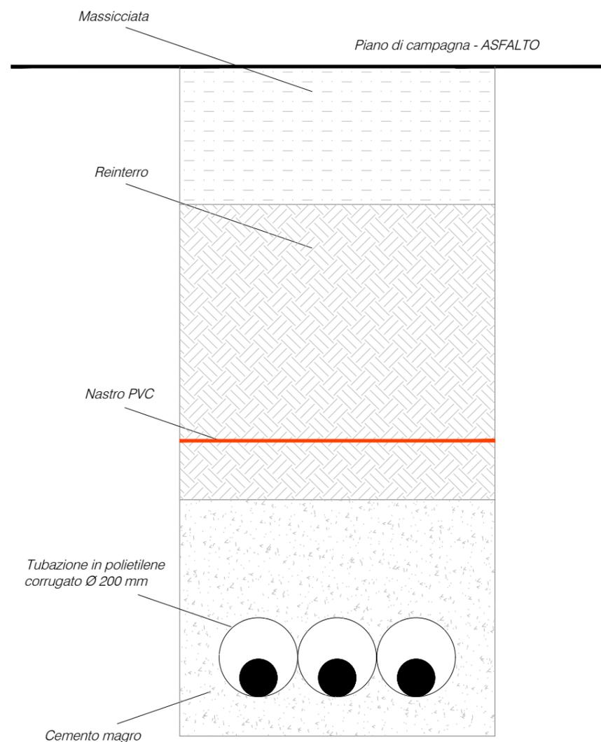
CAVO UNIPOLARE AT 150 kV - ARE4H1H5E 630 mm<sup>2</sup>
