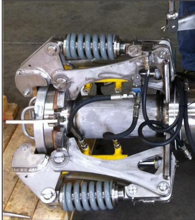
**Figura 15 - Quick Connect / Disconnect Coupler**
