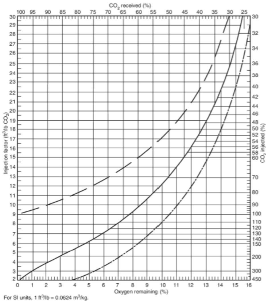
FIGURE D.1(a) Carbon Dioxide Requirements for Inert Atmospheres [based on a carbon dioxide expansion of 9 ft<sup>3</sup>/lb (0.56 m<sup>3</sup>/kg)].
