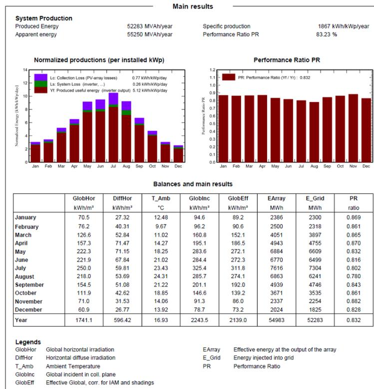
FIGURA 5: PRODUCIBILITA' ELETTRICA DELL'IMPIANTO AGRIVOLTAICO VALUTATA TRAMITE PVSYST
