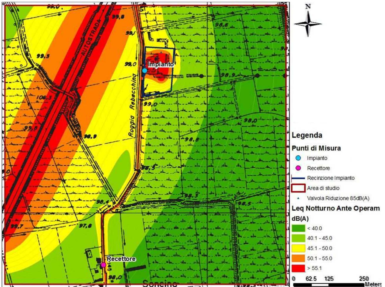
Fig. 9.3 – Leq Notturmo in dBA – Ante Operam
