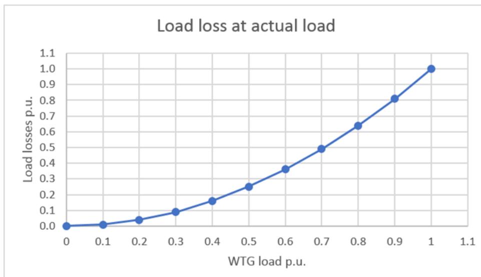
Figure 4-2: Transformer load losses scaling
