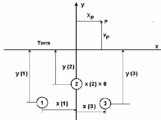
$$B_x = \frac{\mu_0}{2\pi} \sum_i I_i \left[ \frac{y_i - y}{(x - x_i)^2 + (y - y_i)^2} \right]$$
