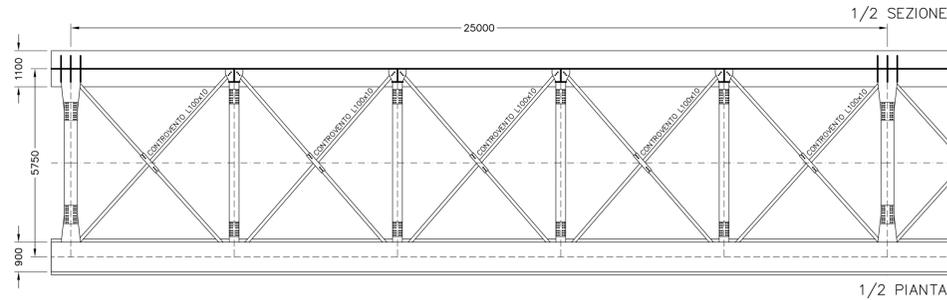
SEZIONE LONGITUDINALE CAMPATA 1 CARREGGIATA DX L=25m SCALA 1:100
