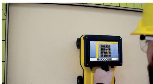
Automatic position and navigation system (Virtual Pad) increases productivity and reduces survey times.
