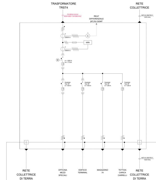
SCHEMA UNIFILARE QUADRO GENERALE BASSA TENSIONE REFEERS
