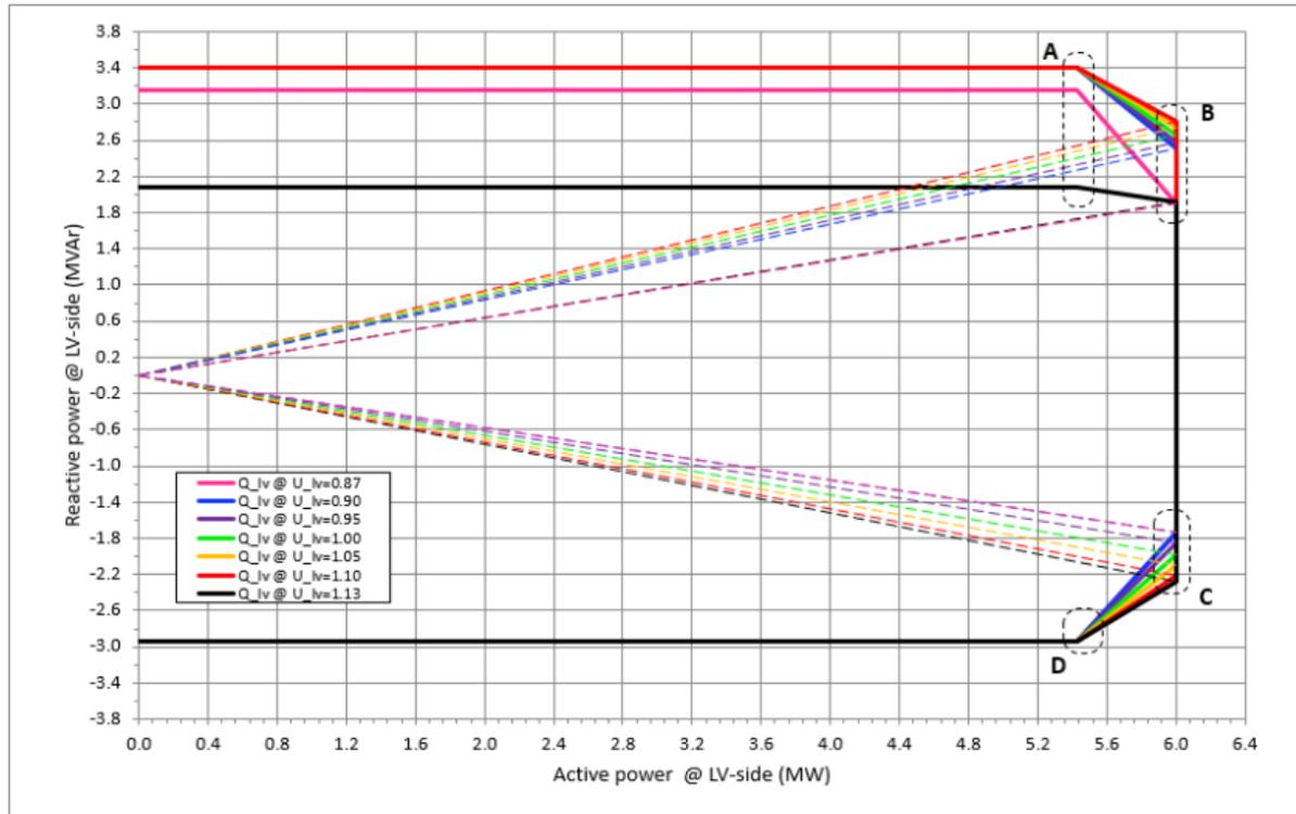
**Figura 1** – Capability aerogeneratori Vestas V150 – 6 MW
