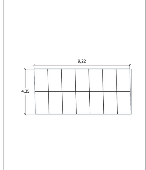
TIPOLOGICO STRUTTURA A UNA STRINGA (2 x 14 MODULI) Scala 1:100
