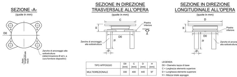
**DISPOSITIVI DI APPOGGIO A DISCO ELASTOMERICO CONFINATO - FISSO**
