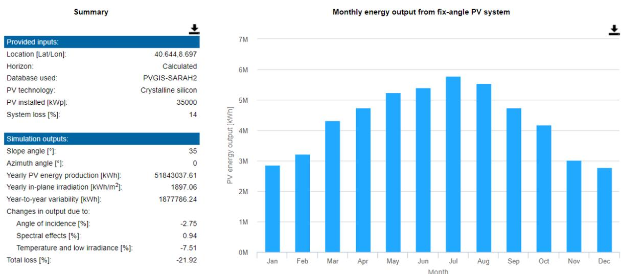
**FIGURA 8: PRODUCIBILITA' ELETTRICA DELL'IMPIANTO FOTOVOLTAICO STANDARD VALUTATA TRAMITE PVGIS**
