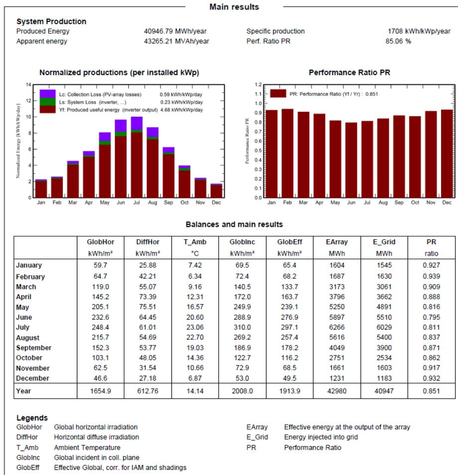
FIGURA 7: PRODUCIBILITA' ELETTRICA DELL'IMPIANTO AGRIVOLTAICO VALUTATA TRAMITE PVSYST
