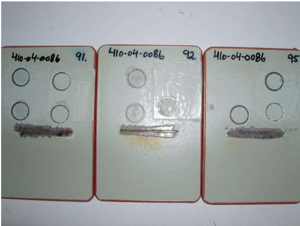
Photo no.1. Panels after the Sea Water Immersion test
