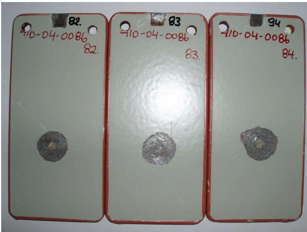
Photo no.2. Panels after the Cathodic Disbonding test
